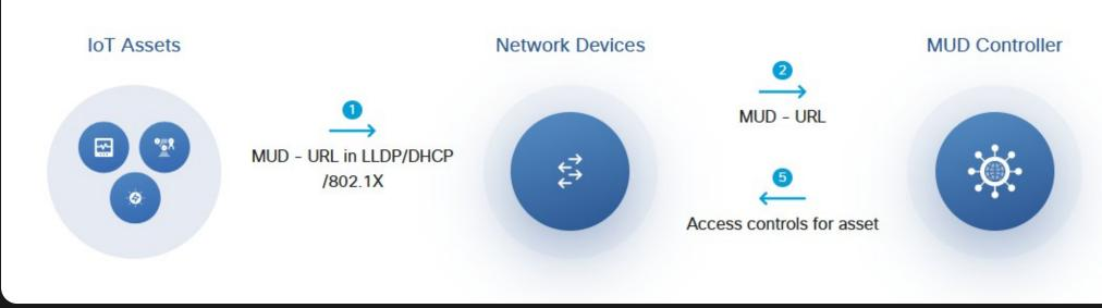
MUD files whitelist the nature of network traffic that a device should transmit/receive. (e.g. Transmit IPv4 tcp/8890 to (DNS) example.com)
